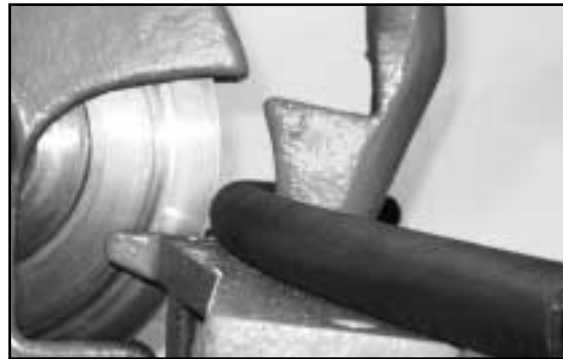
Cut-off saw. Use caution when operating power equipment. Follow the proper safety measures per manufacturer suggestions.
