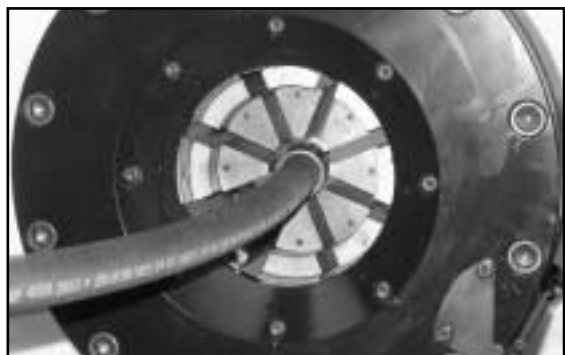
Insert hose assembly into crimper die set.
