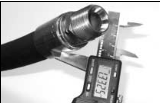
Verify crimp diameter with calipers.
