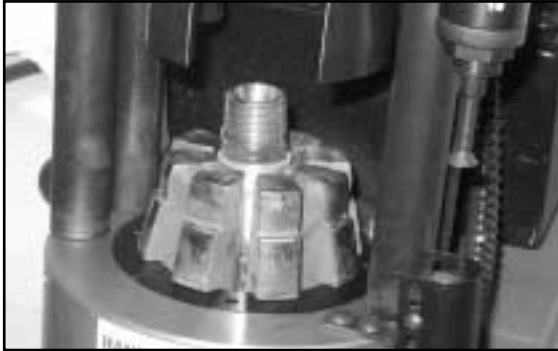
Insert hose assembly into crimper die set.
