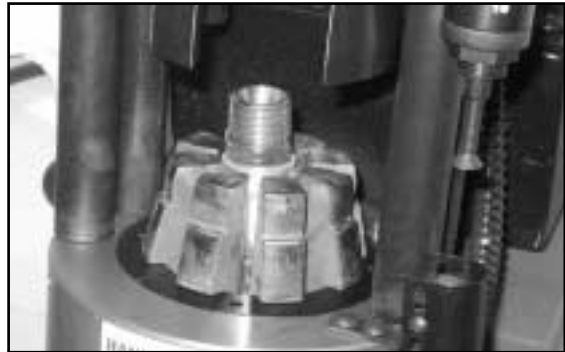
Insert hose assembly into crimper die set.
