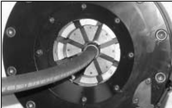
Insert hose assembly into crimper die set.
