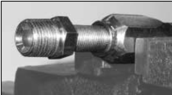
Screw stem into socket.
