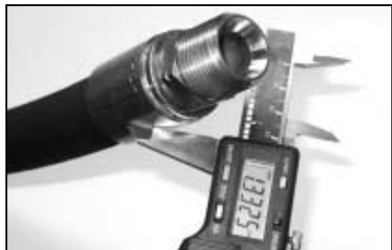
Verify crimp diameter with calipers.
